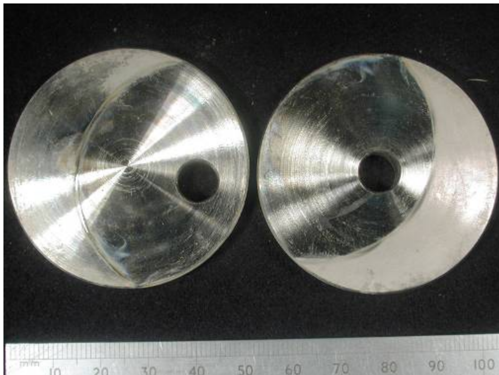
Figure 11. Zeron 100 coupons after test in 500 ppb O 2 , before cleaning.
